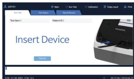
③ Analyzer checks the conditions of the inserted test device. If the test device has already been used, E-1 error pops up.
