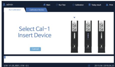
② After checking the Cal-1 Device, insert the Cal-2 Device into the test slot of the Analyzer.
