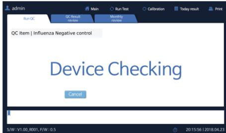
⑤ When the verification of the test device is completed, apply the control to the sample well of the test device and immediately press "QC Start".
