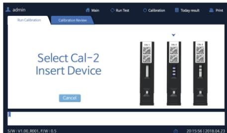
③ After checking the Cal-2 Device, insert the Cal-3 Device into the test slot of the Analyzer.
