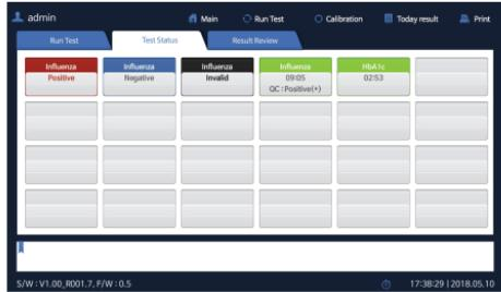
① If you select a completed item, you can check details of the test(test result, name label, procedural control, test date and time, Operator ID, Patient ID, manufacturing date of the test device, software version). In this window, you can print the test result by pressing on "Print". Press "OK" to close the window.
