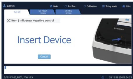
④ The Analyzer checks the conditions of inserted test device. If the test device has already been used, an E-1 error pops up.
