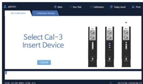
④ After inserting all the calibration devices, the analyzers performs the calibration analysis.
